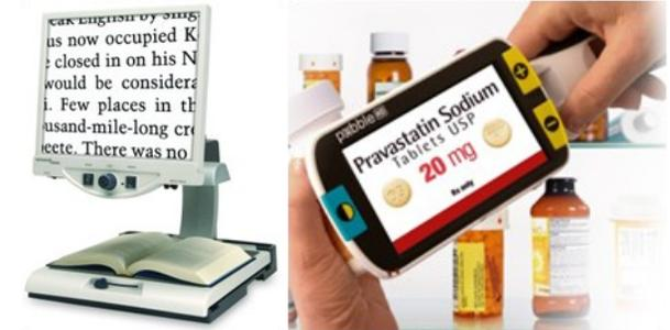
*Video magnifiers, whether desk-top or portable in design, provide variable magnification and the ability to store the text.*
